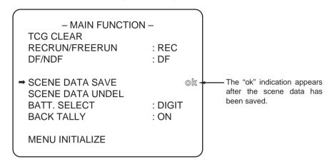
Use the ITEM button to align the arrow with the SCENE DATA SAVE position, and press the UP or DOWN button.
